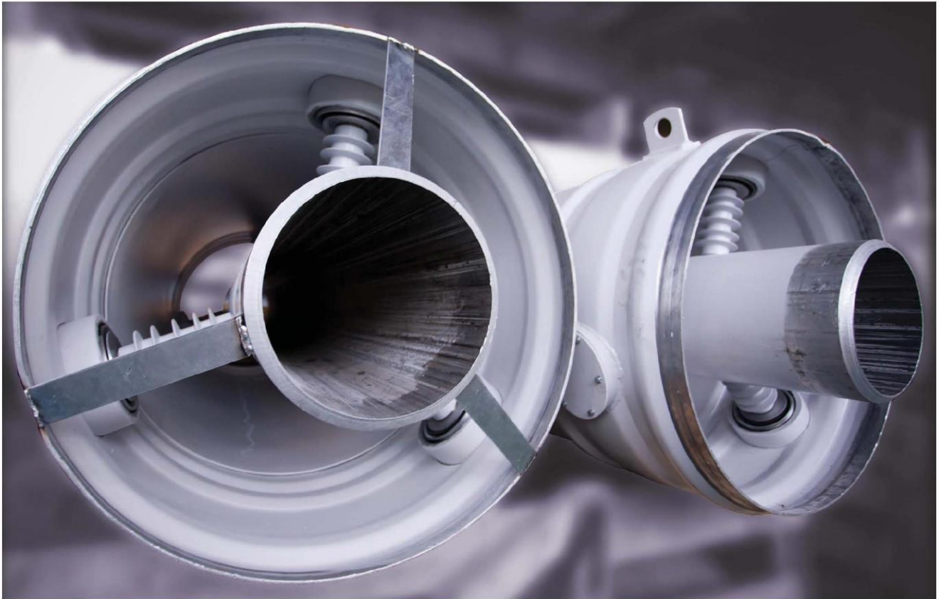
Fig. 6. A view of TENE-20-10000-300UKhL1 busduct's phase, busbar diameter – 280 mm, casing diameter - 750 mm.
